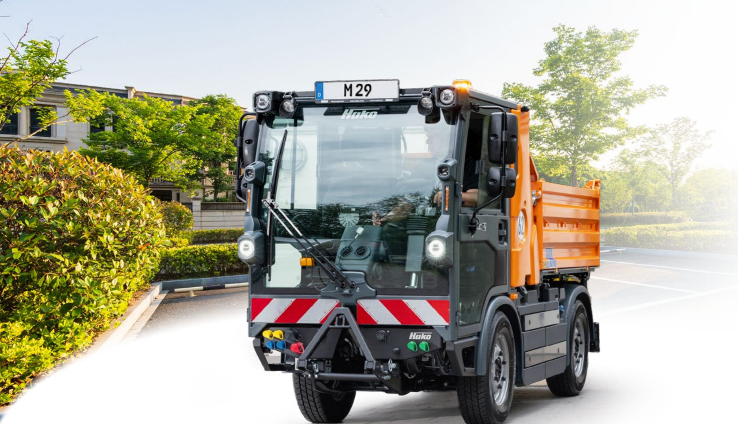
Flexible design as standard: The quick-change systems of the Multicar M29. In the picture: robust attachment triangle for front attachments.
